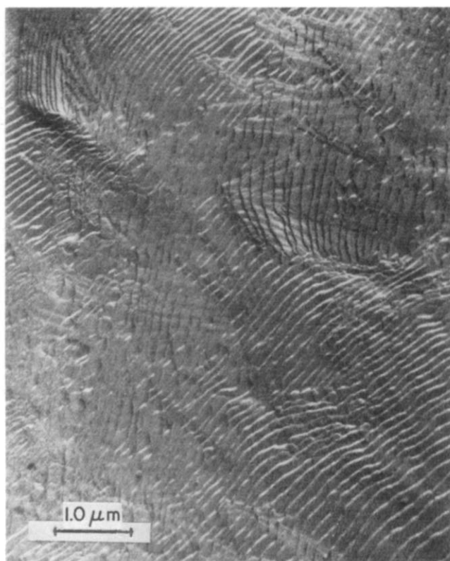
Figure 4 Lamellar microstructure of MW = 9230 PEO fraction crystallized from the melt. The crystallization temperature is 331.7 K
